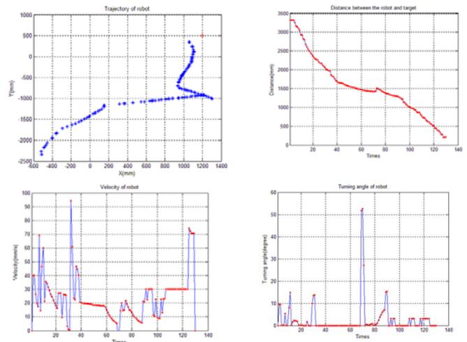
Figure 22. (Top Left) Trajectory of the robot; (Top Right) Distance between the robot and the target; (Bottom Left) Velocity of the robot; (Bottom Right) Turning angle of the robot.
