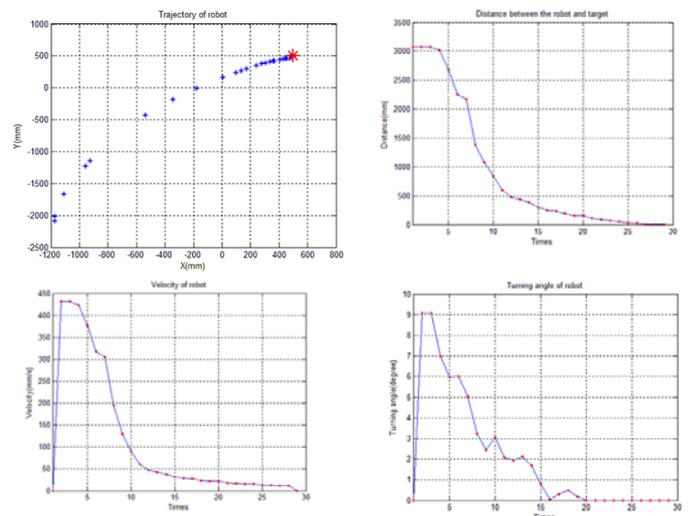
Figure 18. (Top Left) trajectory of the robot; (Top Right) Distance between the robot and target; (Bottom Left) Velocity of the robot; (Bottom Right) Turning angle of the robot.
