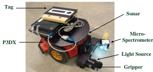
Figure 14. The prototype mobile robotic system.
