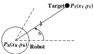
Figure 8. The angle and distance between robot and target.
