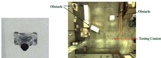
Figure 15. Experimental setup: (Left) Camera on the ceiling; (Right) Photo taken from the camera.
