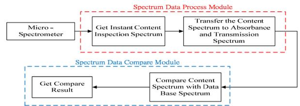
Figure 13. Micro-spectrometer based content identification.
