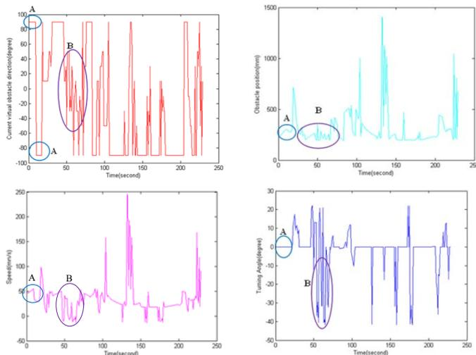
Figure 20. (Top Left) Current obstacle orientation w.r.t. the robot; (Top Right) Obstacle position; (Bottom Left) Velocity of the robot; (Bottom Right) Turning angle of the robot.
