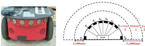
Figure 5. Sonars arrangement: (Left) in mobile robot; (Right) defined configuration.
