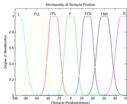
Figure 12. Membership functions for obstacle orientation.
