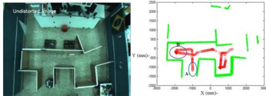
Figure 19. (Left) Maze; (Right) Trajectory of the robot.
