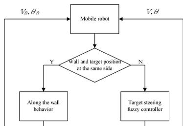
Figure 11. Motion control: left-wall or right-wall.
