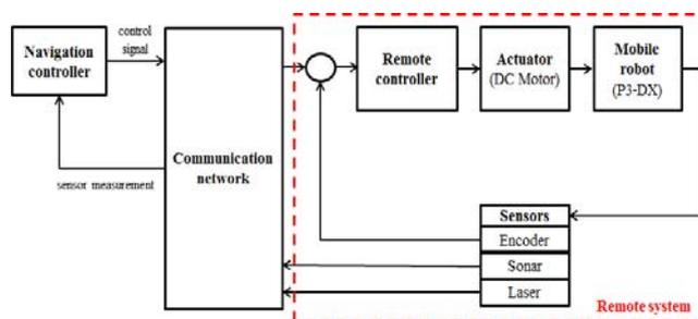
Figure 2. Hierarchical networked control system.
