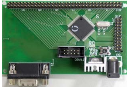
Figure 11. PWM MCU control module.
